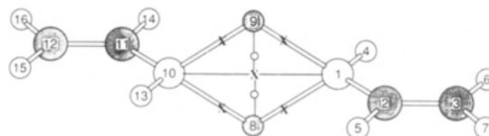
Figure 3. Schematic representation of the topological properties of the \text{Li}_2\text{N}_2 rings in 3a (similar for 4a ). Bond critical points are marked "X" and ring critical points are marked by "O".
